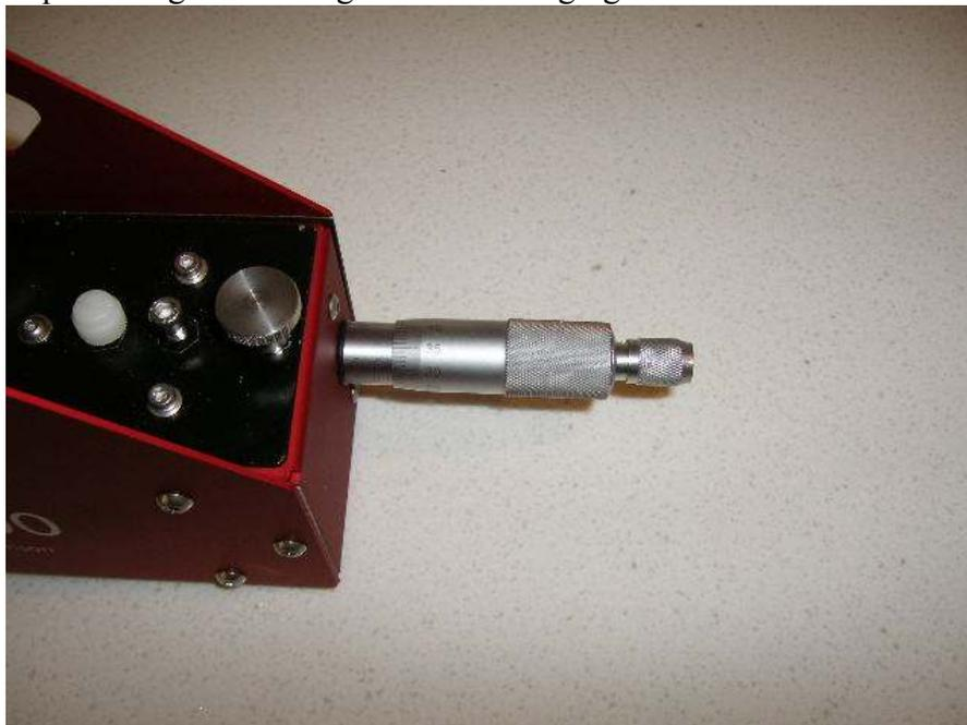
**Fig 11** Grating adjustment micrometer head
