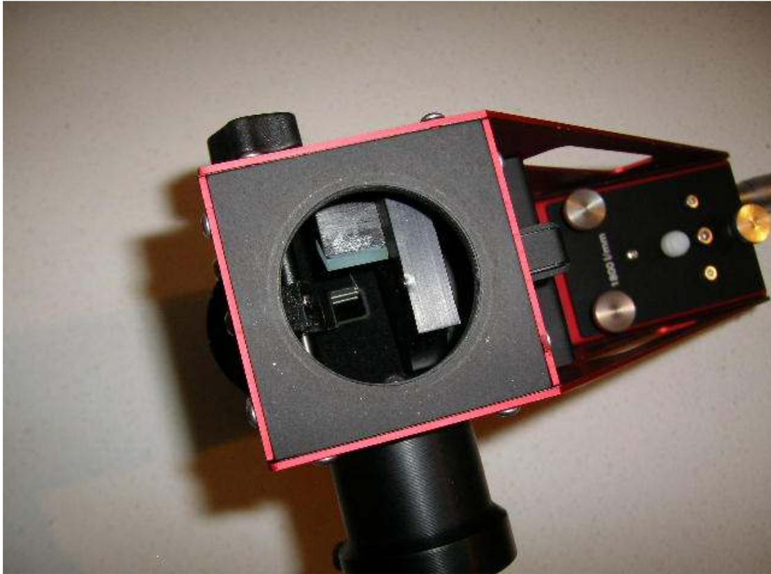
*Fig 3 Inlet port showing slit plate (reference mirror retracted)*
