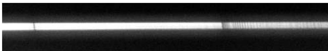
*Fig 15 Spectrum corrected for tilt – showing the slant of the lines within the spectrum\*
