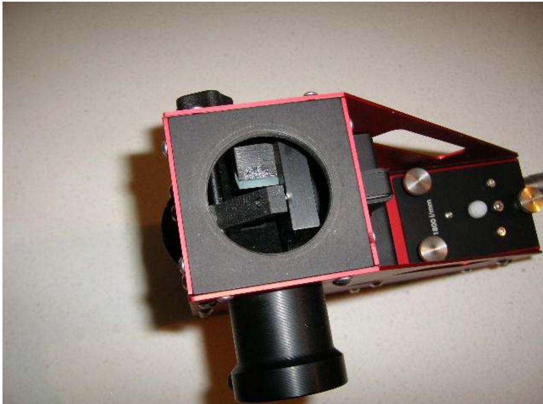
*Fig 6 Inlet port showing reference mirror in position*
