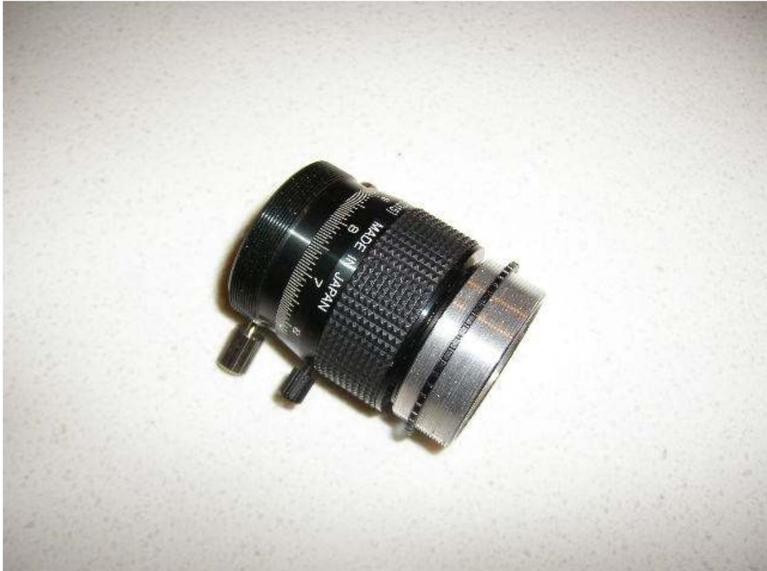
*Fig 17 Borg/Hutech #7315 helical focuser and T thread adaptor*
