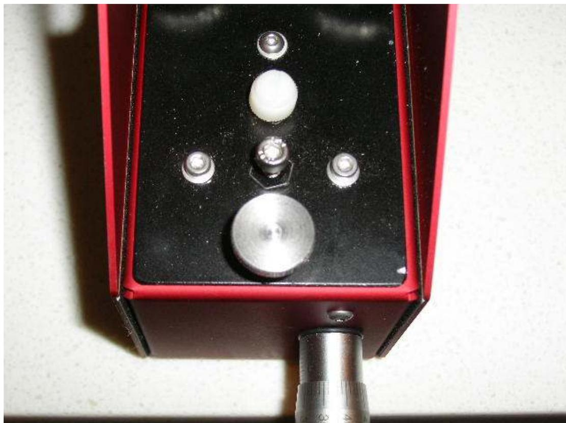
*Fig 34 Grating access cover showing the grating tilt adjust screws*
