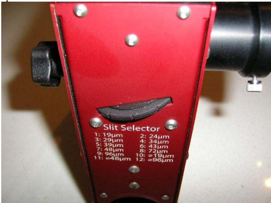
*Fig 4 Thumbwheel indexing for slit gap*
